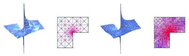
Stokes flow over an L-shaped domain: Pressures and meshes for error tolerance of 5% and unstable finite element pairs (resp. DOFs):  $\mathcal{P}^2$ - $\mathcal{P}^1_d$  (1940),  $\mathcal{P}^1$ - $\mathcal{P}^1$  (4971). The oscillations do not persist under further selective refinement (nonlinear stabilization effect of adaptivity). Error estimation and adaptivity will be fully discussed in this course.
