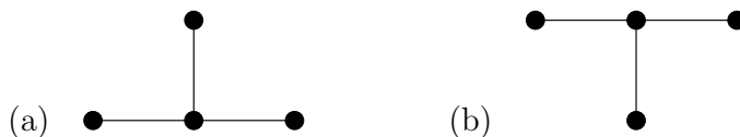
Figure 2.1: (a) The stencil of the Forward Euler method. (b) The stencil of the Backward Euler method.
