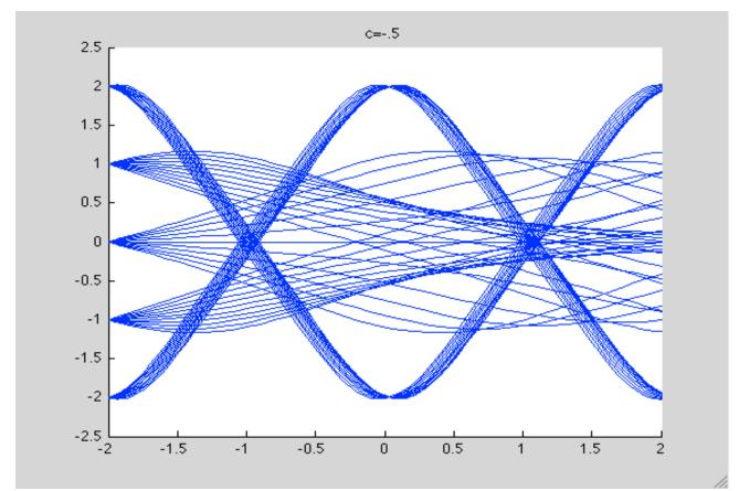
For c= -0.5, the curves from y=2 & y=-2 have the second anti-node a little earlier at x=1.1. The curves from y-1 & y=1 start converging and almost cross at x=2. The curve from y=0 opens up conically, and is at its widest a little earlier at x=0.4 with a decreased amplitude of 1.4, before starting to converge.
