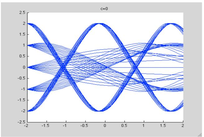
For c= 0.0, the curves from y=2 & y=-2 have the second anti-node just a little before x=0.9. The curves from y-1 & y=1 start converging a little faster and cross right before x=0. The curve from y=0 opens up conically, is at its widest even earlier at x=0.3 with a decreased amplitude of 0.9.
