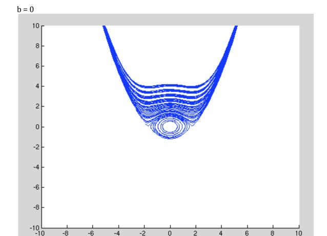
This is the phase diagram for  $x'' + bx' + x - (1/3) x^3 = 0$ . There are three critical points (0,0),  $(-3^{(1/2)},0)$ , and  $(3^{(1/2)})$ . There is a center at (0,0) and the other two points are saddles. The center is stable and the other two are unstable. In order to plot this, I needed to convert the equation into a system of equations where Dx1=x2 and  $Dx2=-bx2-x1+(1/3)x1^3$ .
