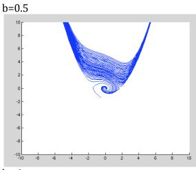
As b increases, the center point becomes a spiral. It is going in the clockwise direction into the origin, so it is becoming into a spiral sink. It is still table and attracting. Due to this direction, the right side appears to have a more defined asymptote.
