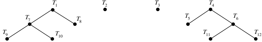
Fig. 3 Forest \mathcal{F}_2 corresponding to the grid sequence \{\mathcal{T}_k\}_{k=0}^2 of Figure 2. The roots of \mathcal{F}_2 from the initial mesh \mathcal{T}_0 and the leaves of \mathcal{F}_2 constitute the conforming bisection mesh \mathcal{T}_2 . Moreover, each level of \mathcal{F}_2 corresponds to all elements with generation equal to the level.
